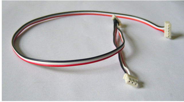
Figure 3-5. IPMB cable
