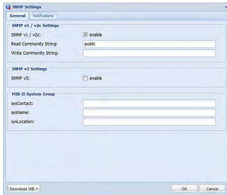
2. Select the "enable" checkbox in the "SNMP v1 / v2c" field to enable communication with an SNMP manager using SNMP v1 or v2c protocol.
