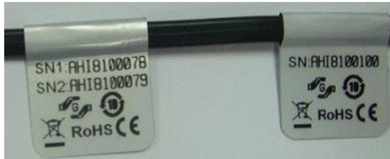
A DPX2 or DX sensor has a serial number tag attached to its rear side.
