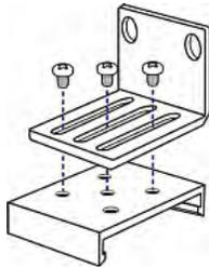
5. Using rack screws, fasten the PX device to the rack through the L-brackets.
