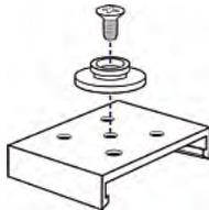
4. Align the large mounting buttons with the mounting holes in the cabinet, fixing one in place and adjusting the other.
