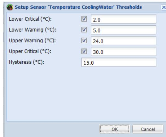
5. Adjust the threshold and deassertion hysteresis settings. The Upper Critical and Lower Critical values are points at which the PX considers the operating environment critical and outside the range of the acceptable threshold.
