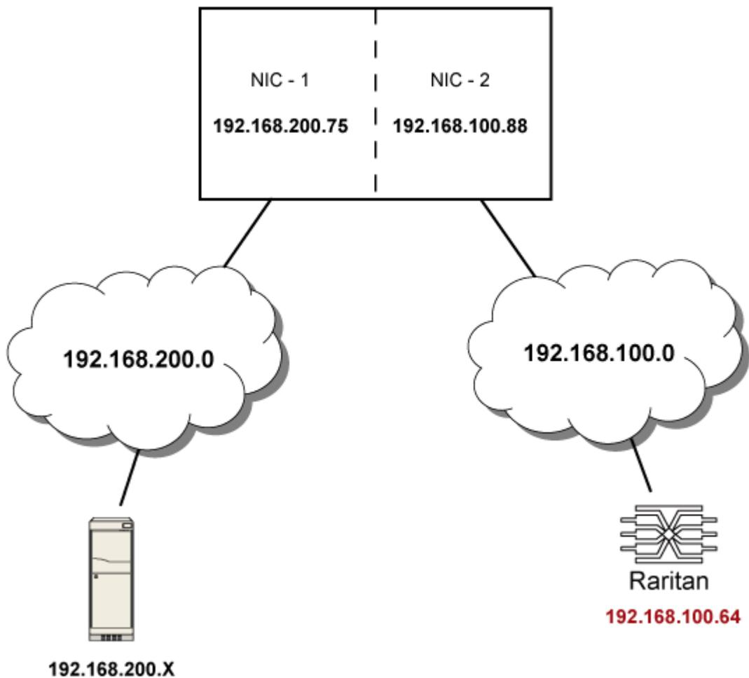
In this example, NIC-2 (192.168.100.88) is the next hop router for your PX to communicate with any device in the other subnet 192.168.200.0. In the IPv4 "Append new Route" dialog, you should specify:
