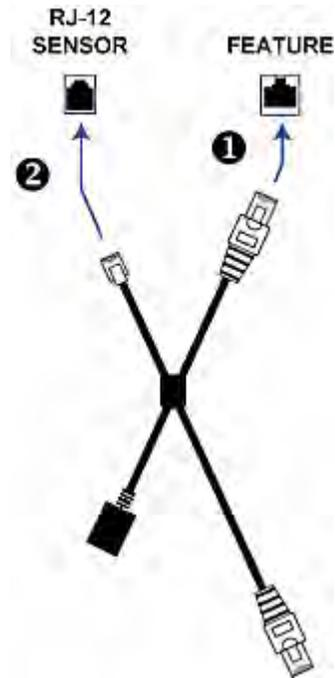
3. Plug the RJ-45 connector at the longer end of the X cable into the RJ-45 port labeled "Input" on the composite asset sensors.
