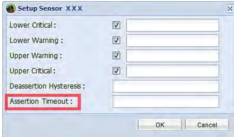
*Note: For most sensors, the measurement unit in the "Assertion Timeout" field is sample. Because the PX measures each sensor every second, timing of a sample is equal to a second.*
