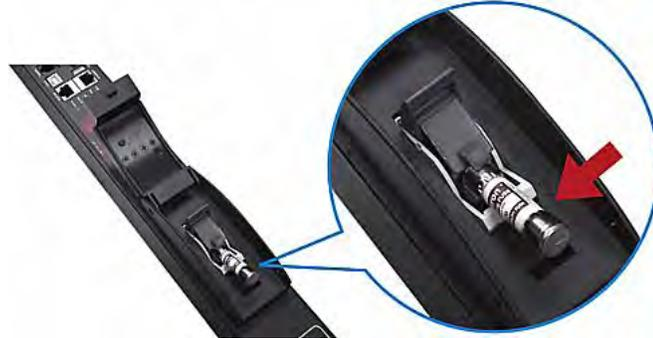
5. Insert a new fuse into the holder. There is no orientation limit for fuse insertion.
