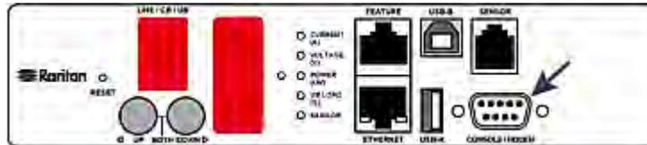
If your computer does not have a serial RS-232 port, use a regular USB cable to connect the PX to the computer for initial configuration. The PX device can emulate a serial port after the USB-to-serial driver is properly installed in the Windows® operating system.
