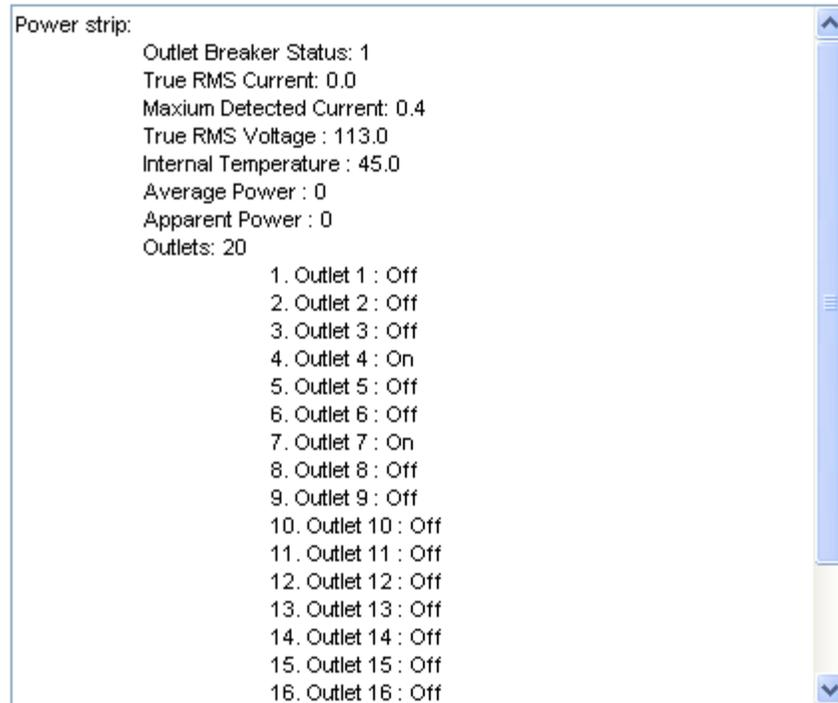
2. A status box appears, displaying details of the controlled PX, including power state of each outlet on the device.
