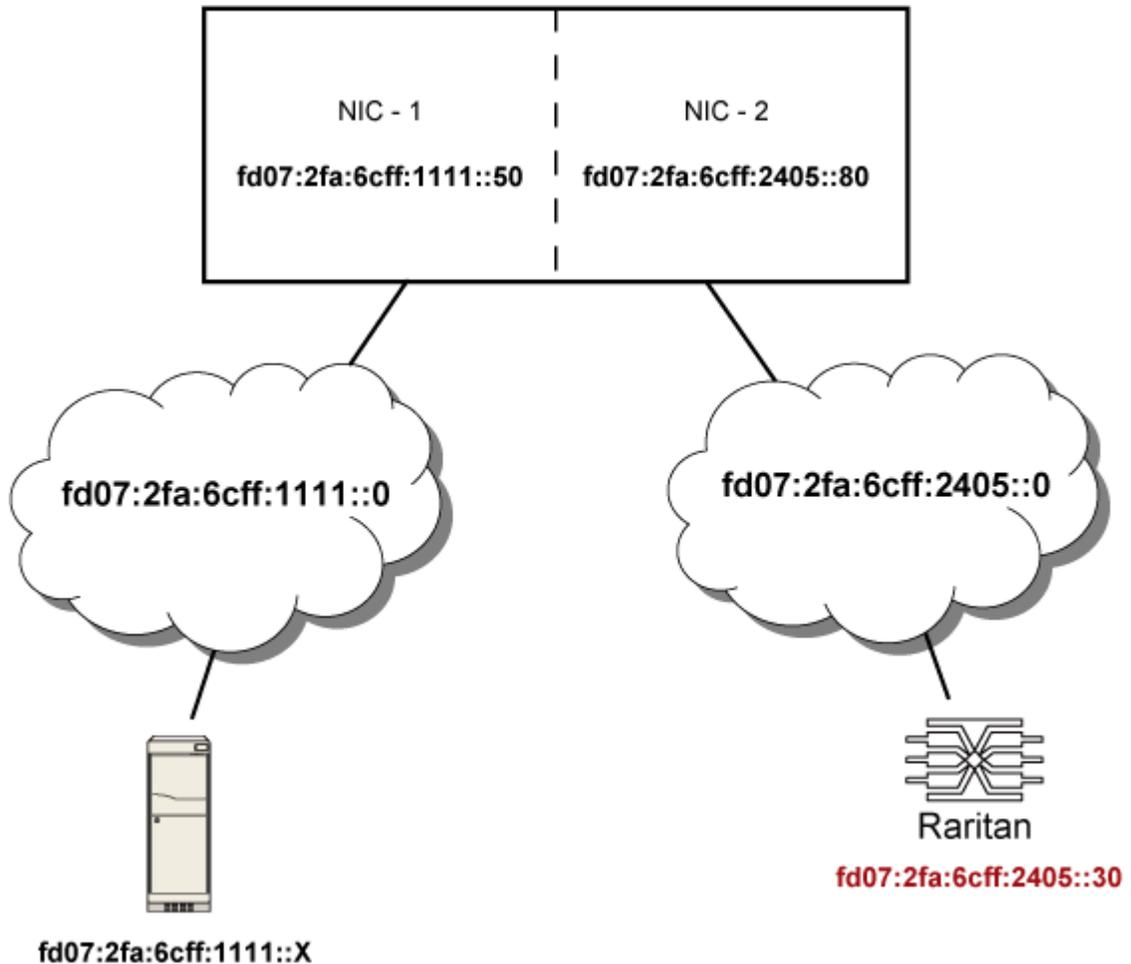
In this example, NIC-2 (fd07:2fa:6cff:2405::80) is the next hop router for your PX to communicate with any device in the other subnet fd07:2fa:6cff:1111::0. In the IPv6 'Append new Route' dialog, you should specify:
