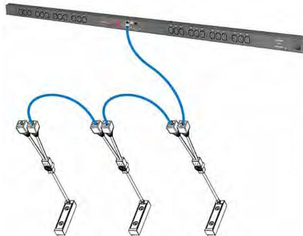
4. Repeat Step 2 to connect IT devices to the other composite asset sensors in the chain.
