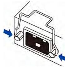
3. Connect the power cord to the inlet, and press the clip toward the power cord until it holds the cord firmly.
