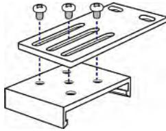
5. Using rack screws, fasten the PX device to the rack through the claw-foot brackets.
