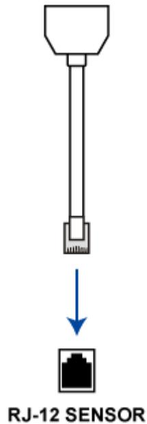
2. A Y cable has two RJ-12 sensor ports. Connect DPX sensor packages to the Y cable's sensor ports.
