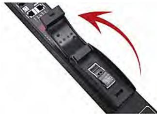
2. Verify the new fuse's rating against the rating specified in the fuse holder's cover.
