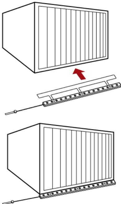
3. Connect one end of an asset tag to a blade server and connect the other end to the blade extension strip.
