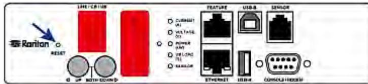
This diagram shows the location of the reset button on 1U models.
