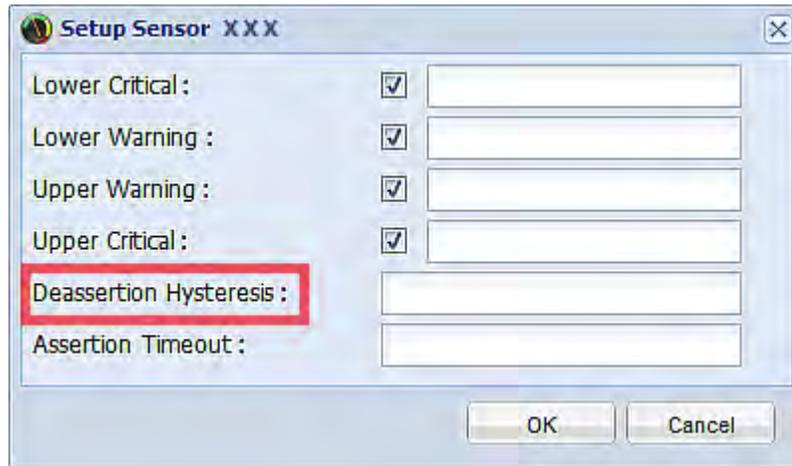
This function is similar to a thermostat, which instructs the air conditioner to turn on the cooling system when the temperature exceeds a pre-determined level. "Deassertion Hysteresis" instructs the PX to de-assert the worse state for a sensor only when that sensor's reading hits the pre-determined "deassertion" level.
