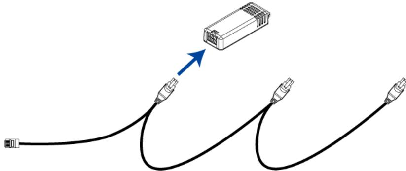
2. Connect remaining DPX2 sensors to the second and then the third head connector.
