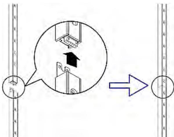
2. Connect another 8U slave asset sensor to the one being attached to the master asset sensor in the same manner as Step 1.
