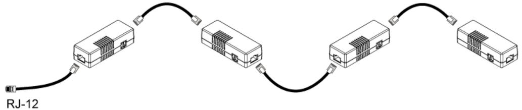
3. Connect the first DX sensor package to the PX.
