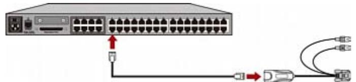
2. Depending on the CIM model you purchased, plug the connectors of the CIM into a server's PS/2 or USB keyboard, mouse, and VGA ports.
