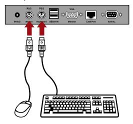
Note: Do NOT connect both of PS/2 and USB keyboards or both of PS/2 and USB mice simultaneously. If you do so, only the USB input devices work properly.
