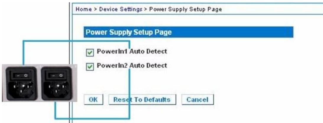
2. If you are plugging power input into power supply number one (left-most power supply at the back of the unit), then select the PowerIn1 Auto Detect option.
