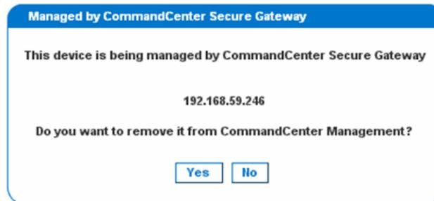
2. Click Yes to begin the processing of removing the device from CC-SG management. A confirmation message will then displayed asking you to confirm that you want the remove the device from CC-SG management.
