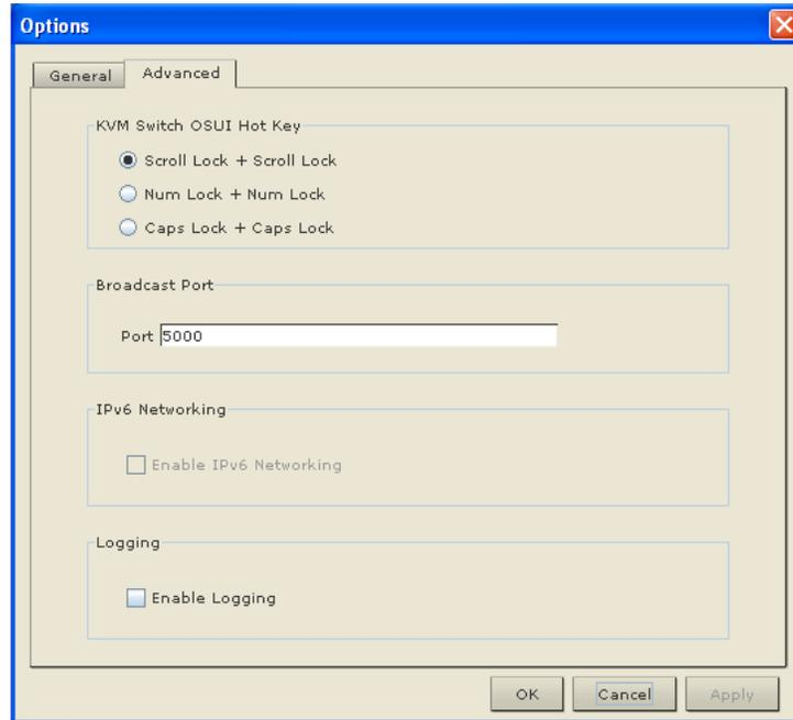
9. From the KVM Switch OSUI Hot Key section, select the hot key to use when switching between target server displays.
