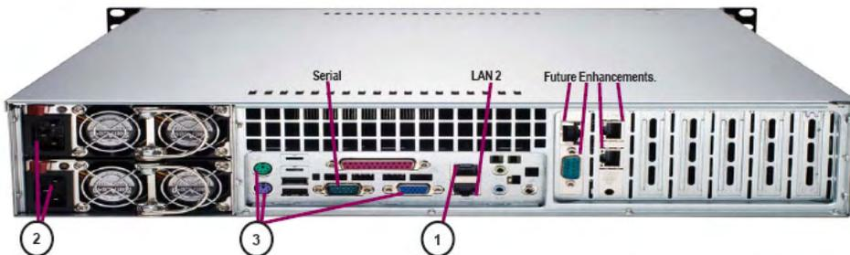
1. Connect the CAT 5 network LAN cable to the LAN 1 port on the rear panel of the CC-SG unit. Connect the other end of the cable to the network.
