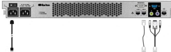
1. Connect the network LAN cable to the LAN 0 port on the rear panel of the CC-SG unit. Connect the other end of cable to the network.
