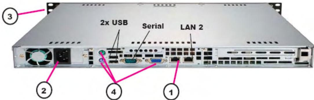
1. Connect the network LAN cable to the LAN 1 port on the rear panel of the CC-SG unit. Connect other end of cable to the network.
