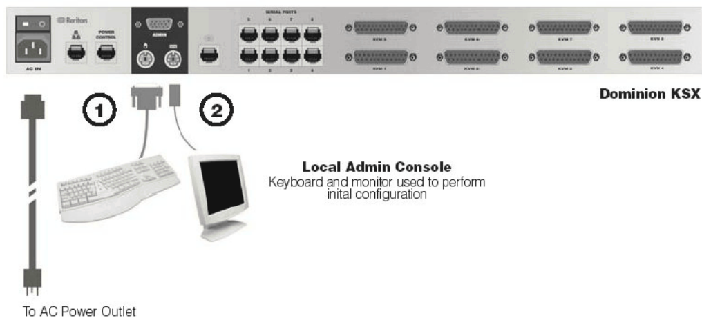
Figure 5: Dominion KSX Back Panel Connections
