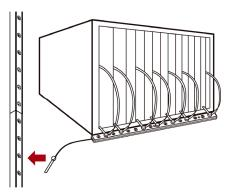
Note: If you need to temporarily disconnect the tag connector of the blade extension strip, wait at least 1 second before connecting it back, or the Raritan SNMP gateway may not detect it.
