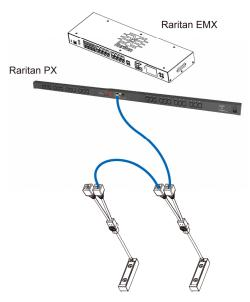
Repeat Step 2 to connect IT devices to the other AMS-M2-Z's in the chain via the asset tags.
